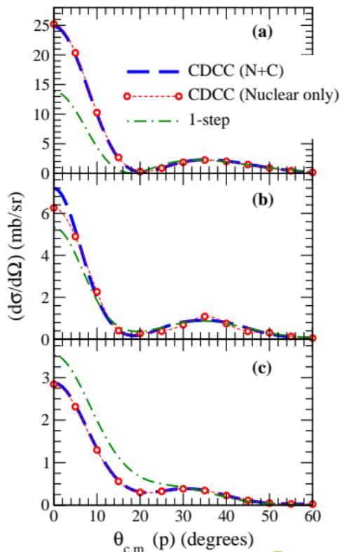
Transfer cross section for deuterons on  $^{10}\text{Be}$  at: (a.)  $E_d = 21.4$  MeV, (b.)  $E_d = 40.9$  MeV and (c.)  $E_d = 71$  MeV.
