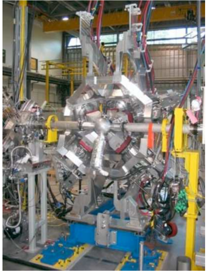
FIG. 1: Arrangement of the HPGe clovers of the TIGRESS array around the target chamber at the end of the ISAC-II beam line at TRIUMF. In this experiment the array comprised six 32-fold segmented clovers. The ^{110}\text{Pd} -target foil and Si-based BAMBINO are mounted inside the chamber.
