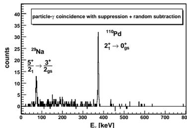
FIG. 1:  $\gamma$ -ray spectrum for  $^{110}\text{Pd}(^{29}\text{Na}, ^{29}\text{Na}^*)$  at  $E_{\text{lab}}(^{29}\text{Na}) = 70$  MeV with a beam intensity of up to  $\sim 600$  pps; the particle angular coverage was between  $20.1^\circ - 49.4^\circ$ .
