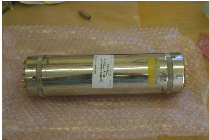
Fifty-plate fission chamber containing ^{235}\text{U} and ^{239}\text{Pu} samples for tagging fission events. This chamber was made at Bruyeres-le-Chatel
