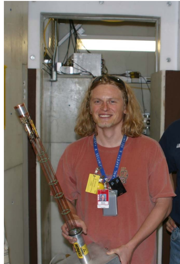
PPAC Assembly with gas lines and signal cables ready for insertion into DANCE center
