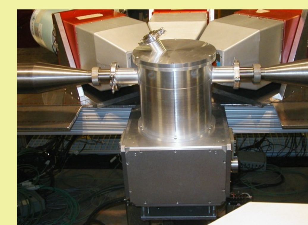
(above) A picture of the STARS chamber, sealed, attached to the beam line at the Lawrence Berkeley National Laboratory. Also shown are half of the Liberace detectors which surround the chamber at varying angles. A schematic drawing of the inside of the chamber is shown on the left.
