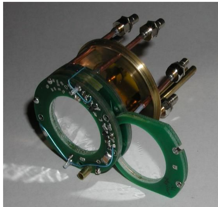
PPAC is customized to fit in the beampipe
